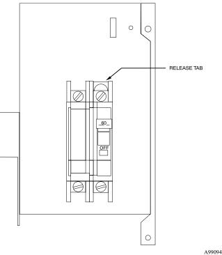
Fig. 17 - Conversion of Circuit Breaker
