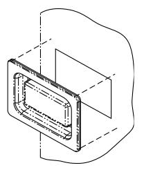
Fig. 4 – Installation of Window Bezel for Circuit Breaker Model Heater
