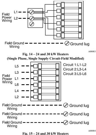
(Single Phase, Multiple Supply Circuits-Field Modified)
