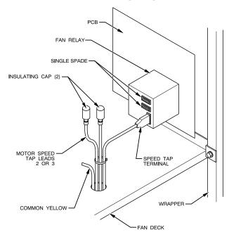
Fig. 16 – PSC Motor Speed Tap and Fan Relay
